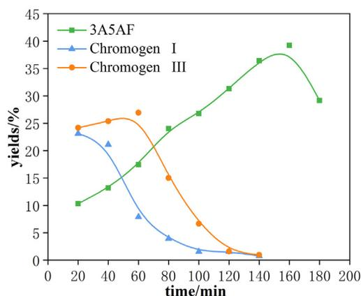
**Figure 5. Effect of reaction time on intermediate and 3A5AF yield**
