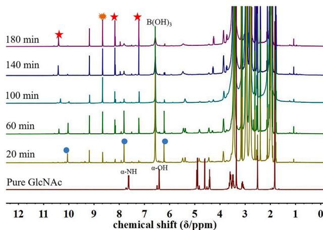
**Figure 3.** *In situ*  $^1\text{H}$  NMR spectra of GlcNAc promoted by  $\text{ChCl-B(OH)}_3$  in DMA at  $140^\circ\text{C}$  for 3 h
