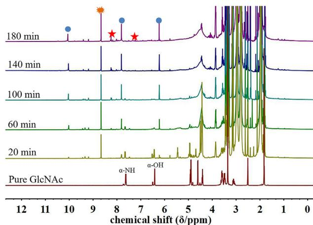
**Figure 1.** *In situ*  $^1\text{H}$  NMR spectra of GlcNAc promoted by ChCl-Gly in DMA at  $140^\circ\text{C}$  for 3 h. Notes: ● Chromogen III, ★ 3A5AF, ✨ Pyrazine
