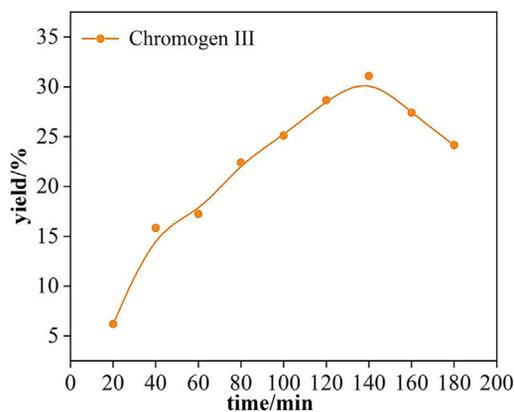
**Figure 2.** Effect of reaction time on Chromogen III yield under normal atmospheric reflux
