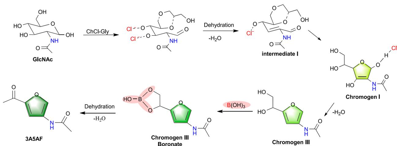
**Scheme 2.** Proposed reaction pathways for the formation of 3A5AF from GlcNAc dehydration
