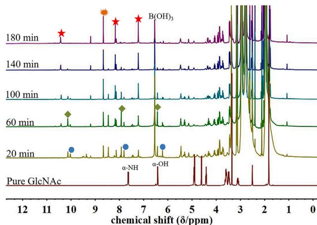
**Figure 4.** *In situ*  $^1\text{H}$  NMR spectra of GlcNAc dehydration mediated by  $\text{ChCl-Gly-B(OH)}_3$  in DMA at  $140^\circ\text{C}$  for 3 h
