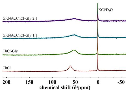
**Figure 7.** The  $^{35}\text{Cl}$  NMR spectra of ChCl, ChCl-Gly, GlcNAc: ChCl-Gly (1:1) and GlcNAc: ChCl-Gly (2:1) in  $\text{DMSO-}d_6$  at  $25^\circ\text{C}$
