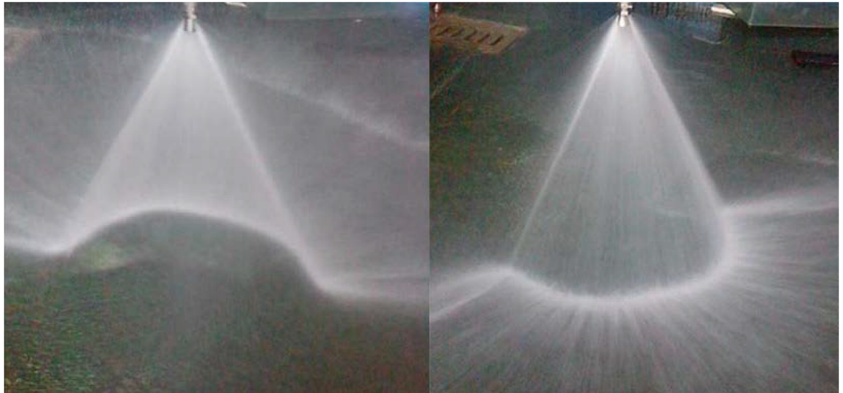
Fig 5. The water spraying effect of the arc fan nozzle.
