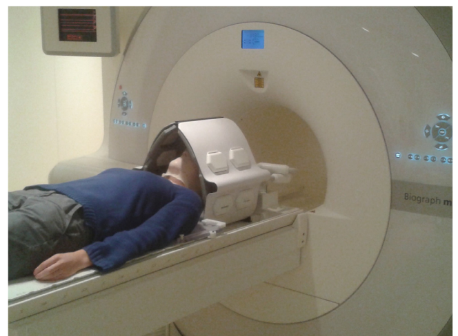
Fig. 2. Dedicated positioning solution for MR imaging of head and neck cancer patients in RT treatment position. The components are a flat table top with an add-on for the fixation of a head and neck positioning mask, and coil holders to which flexible RF coils can be attached.
