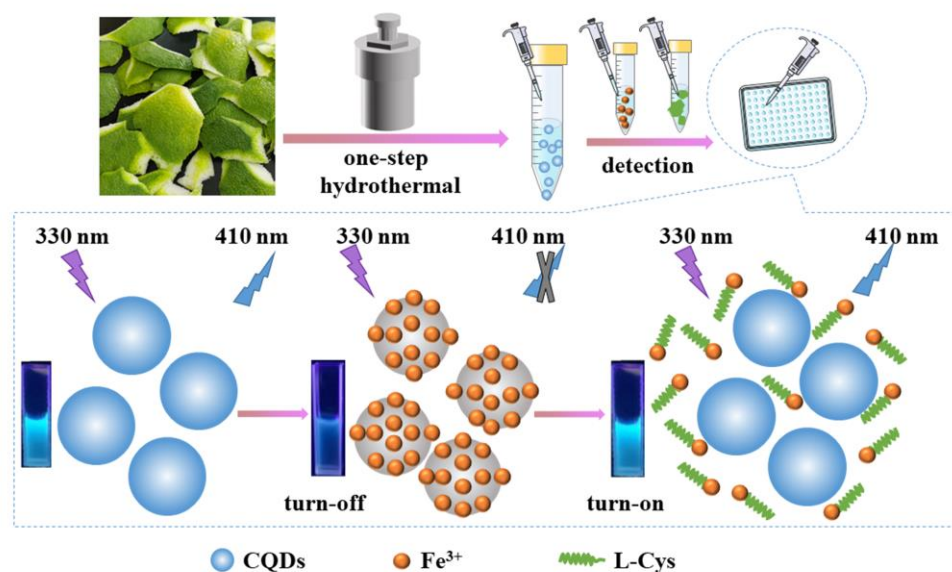
Scheme 1. The detection principle for \text{Fe}^{3+} and L-Cys based on CQDs.
