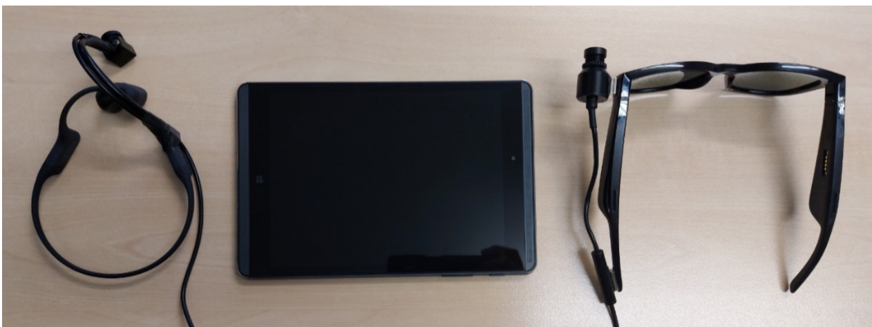
Figure 8. Two realizations of the Colorophone 2.0 system together with the processing unit in the form of a Windows tablet.
