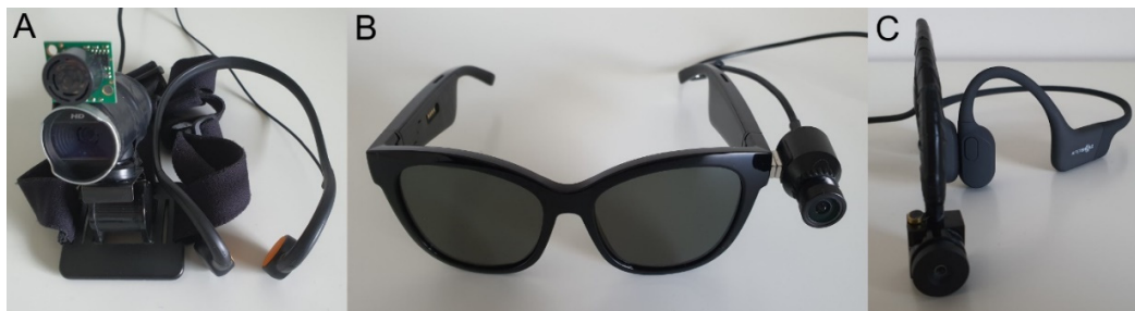
Figure 1. Subsequent versions of the Colorophone system: (A) Colorophone 1.0 with a camera mounted on the headband and headphones; (B) Colorophone 2.0 with Bose Bluetooth audio sunglasses; (C) Colorophone 2.0 with Aftershokz bone-conducting headphones.
