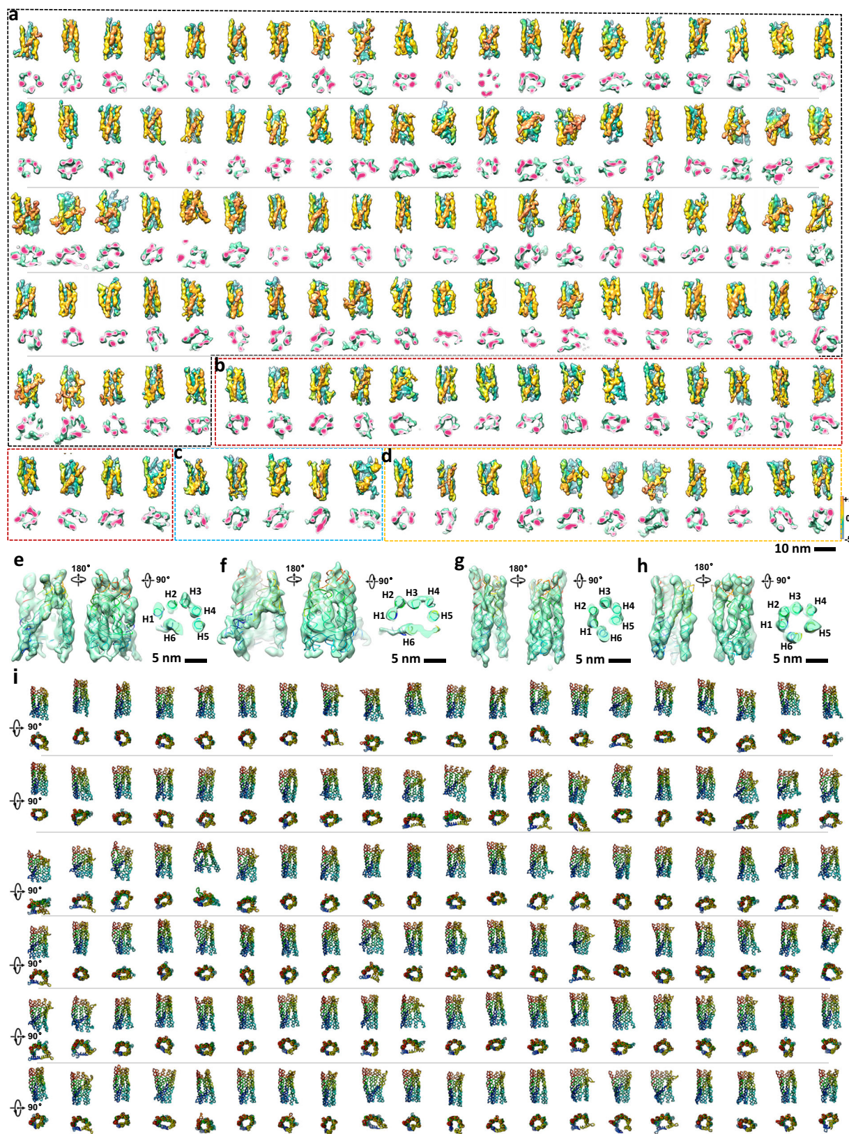
Fig. 4 | A gallery of 120 IPET 3D reconstructions and corresponding fitting models of RNA origami 6HBC. a A total of 85 IPET 3D density maps were reconstructed at a total electron dose of 168 \text{ e}^{-}\text{\AA}^{-2} . b Nineteen maps reconstructed at a dose of 120 \text{ e}^{-}\text{\AA}^{-2} . c Five maps reconstructed at a dose of 107 \text{ e}^{-}\text{\AA}^{-2} . d Eleven maps reconstructed at a dose of 54 \text{ e}^{-}\text{\AA}^{-2} . e, f Two representative young-like particles with
