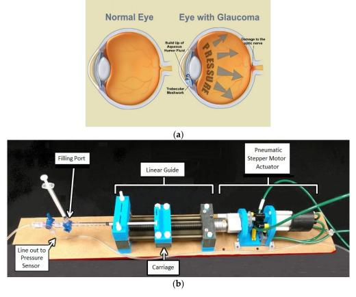
**Figure 1.** (**a**) The effects of glaucoma illustrated [11]. (**b**) A broadly labeled image of the microinjector system setup with syringe.
