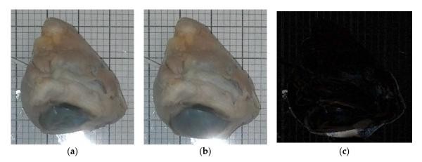
**Figure 3.** (a) (t = 0 s) (pressure = 0 mmHg) (volume injected = 0 mL), (b) (t = 535 s) (pressure = 100 mmHg) (volume injected = 1.75 mL), (c) absolute difference of (a,b). Light region encompassing eye indicates inflation.
