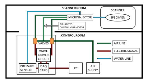
**Figure 2.** The microinjector is placed near or inside the bore of the magnetic resonance imaging (MRI) scanner. The control box, PC, and air compressor are in the control room, connected to the system as shown.
