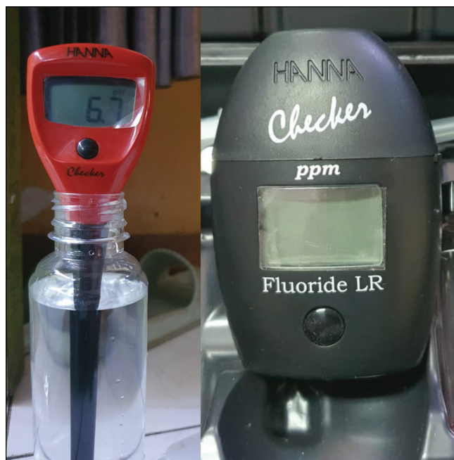
Figure 1: pH Meter and Fluoride Low Range Tool (HI729) Kit. pH Meter (left) and Fluoride Low Range Tool (HI729) Kit was used for analyzing the mineral contents and pH of drinking water and diluted saliva in this study
