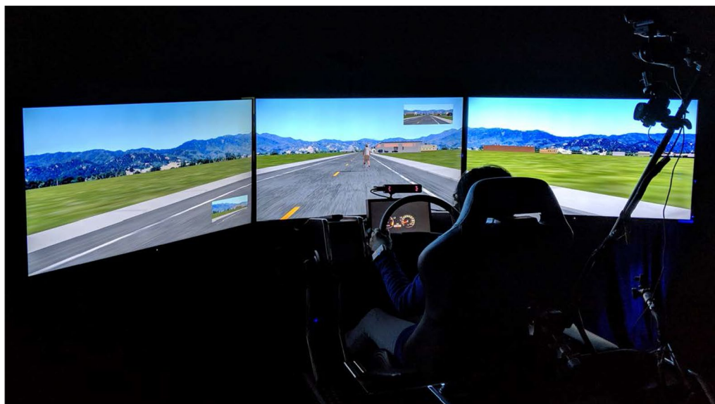
Fig. 1 Driving simulator apparatus. *This figure was published in Goddard et al. (2020), Copyright Elsevier 2020. Reprinted with permission
