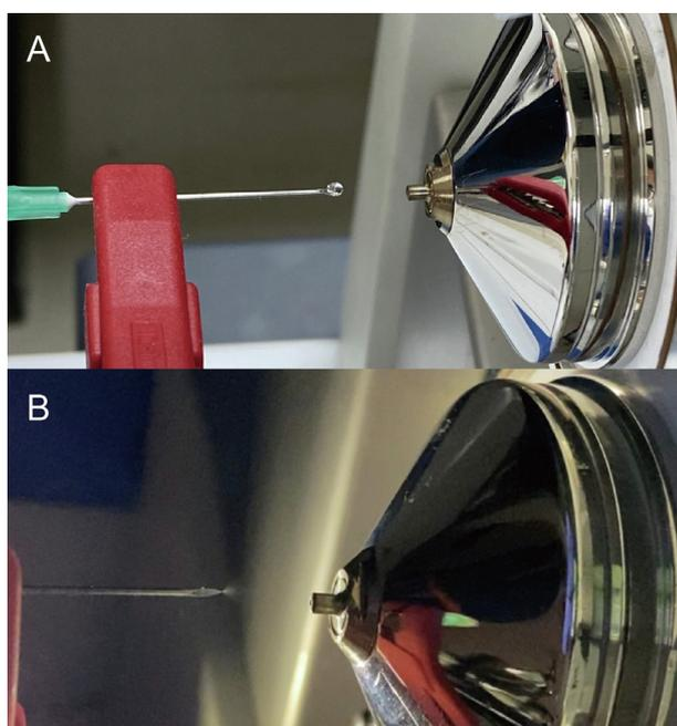
**Fig. 2.** Electrospray ambient ionization mass spectrometry (ESI-AIMS) analysis of saliva using (A) dilute-and-shot mode and (B) extraction and online elution.
