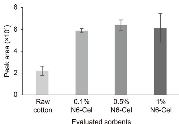
**Fig. 3.** Effect of the amount of polyamide in nylon 6-cellulose (N6-Cel) composite on the extraction performance. The results are obtained by the offline elution of the analyte and its analysis by direct infusion coupled to tandem mass spectrometry (DI-MS/MS), but the same trend is observed for ambient ionization mass spectrometry (AIMS) analysis. The error bars represent the standard deviation obtained for 3 replicates.
