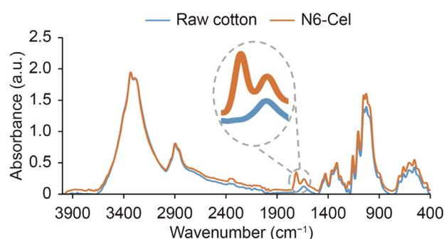
**Fig. 4.** Attenuated total reflection infrared spectroscopy (ATR-IR) characterization of the sorbent, where the spectra of raw cotton and nylon 6-cellulose (N6-Cel) are compared.
