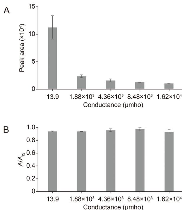
**Fig. 5.** Effect of the ionic strength (expressed as conductance) on the extraction performance using (A) the absolute signal of the analyte and (B) the signal normalized by the internal standard (IS). The error bars represent the standard deviation obtained for 3 replicates.
