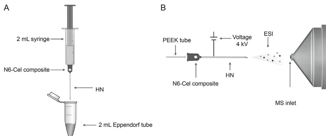
**Fig. 1.** Schematic diagram of the (A) extraction and (B) ambient ionization mass spectrometry (AIMS) analysis using modified hypodermic needles. N6-Cel: nylon 6-cellulose; HN: hypodermic needle; PEEK: polyether ether ketone; ESI: electrospray; MS: mass spectrometry.
