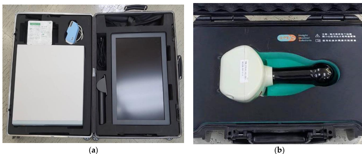
Figure 1. (a) Image processor, LCD monitor and InsightEyes EGD, packed in a roller suitcase. (b) Hand-held magnetic field navigator.
