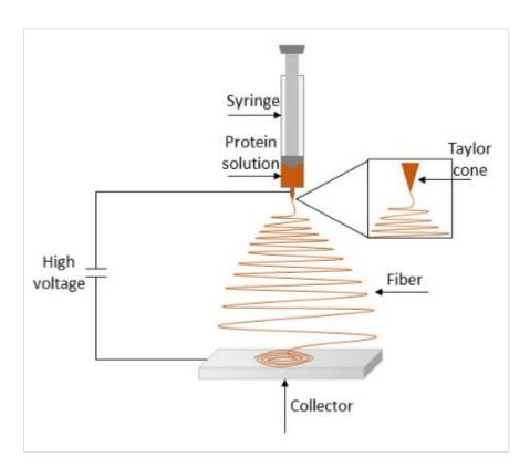
Figure 3. Principle and typical setup of electrospinning.
