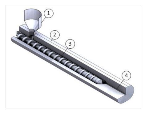
**Figure 2.** Co-rotating twin-screw extruder scheme. (1) Feed (2) Barrel (3) Left screw (right screw mostly hidden) (4) Cooling die.
