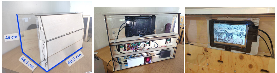
Figure 3. The enrichment device. Left: measurements from the outside, Middle: with the side panel removed to show the technology and screen, Right: view of the screen with the camera below from inside the system.
