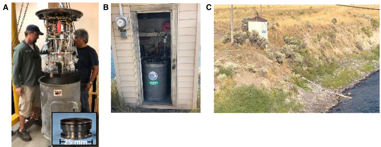
Figure 1. The ESP is an electro-mechanical robot that can autonomously filter and preserve samples. (A) About the size of a 50-gal barrel, the ESP carries 132 ‘pucks’ (inset), each designed to hold 25 mm filters. (B) The ESP installed in a USGS streamgage station. (C) Streamgage station showing tubing run (white pipe) that contained pump and tubing to deliver stream water to the ESP. The ESP communicated via cell phone, and was powered during the deployment via either line power or portable solar arrays. Photo credits: U.S. Geological Survey.
