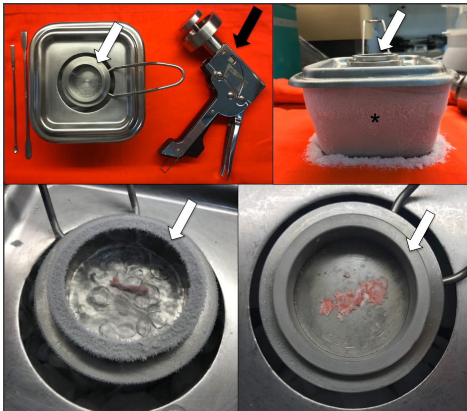
Figure 2. Device composed of a larger lower metallic reservoir (asterisk) where dry ice is placed and a smaller upper metallic reservoir (white arrow) where femoral bone homogenate is obtained through manual shots with a specific pistol (black arrow).
