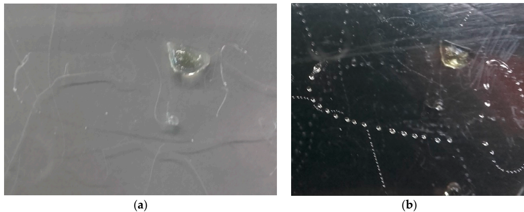
Figure A1. Fibres drawn from a carbohydrate glass solution directly after and 24 h later (a) Intact fibres of carbohydrate glass in random shapes and sizes; (b) Same fibres but now 24 h later. Fibres are mostly dissolved into droplets with only the larger pieces of carbohydrate glass still recognisable.
