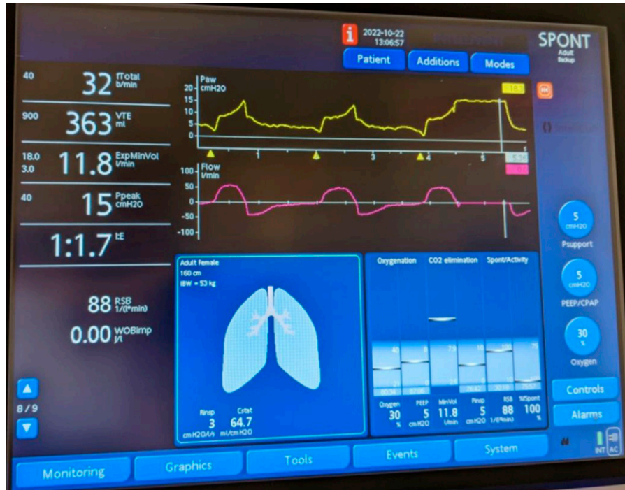
Figure 2. True driving pressure on pressure support ventilation. On the Hamilton-G5 ventilator, patient is on pressure support of 5 cm H 2 O on positive end-expiratory pressure of 5 cm H 2 O. When an end-inspiratory hold maneuver is performed, plateau pressure is found to be at 18 cm H 2 O (top right of image). This translates to the patient exerting an additional 8 cm H 2 O of negative pressure ( P_{mus} = 8 ) to the expected 5 cm H 2 O of pressure support, to generate their tidal volume of 363 ml. The true driving pressure is 13 cm H 2 O. PEEP = positive end-expiratory pressure; P_{mus} = difference between plateau pressure and peak pressure; P_{support} = Pressure support.
