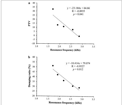
**Fig. 3** The relationship between the resonance frequency of the tested tooth model and the **a** periotest value and **b** damping ratio. A high correlation was found between the readings of resonance frequency and damping ratio
