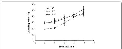
**Fig. 6** Changes in the damping ratios of the models with various root types and degrees of bone loss. *UCI* upper central incisor, *UFP* upper first premolar, *UFM* upper first molar
