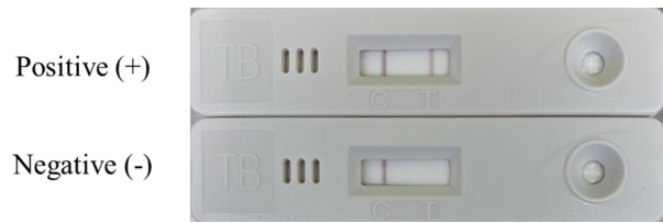
Fig. 1 – Positive, clear and distinguishable red bands appear in both the control (C) zone and the test zone (T). Negative, only one red band appears in the control (C) zone.
