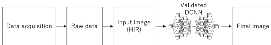
Fig. 2 Flowcharts of the training and reconstruction process in deep learning reconstruction (DLR). a In the training process, given standard-dose images by hybrid iterative reconstruction (HIR) as low-quality input data and high-dose images by advanced model-based iterative reconstruction (MBIR) with much more iterations than MBIR as targeting high-quality data as training pairs, the deep convolu-
