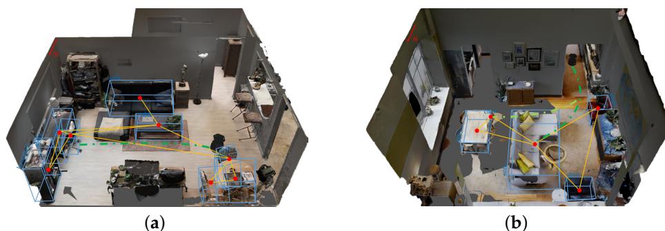
Figure 1. Illustration of the proposed object-level topological path planning for visual navigation. (a,b) shows two different indoor scenarios. The blue boxes represent the 3D object detection of object-level landmarks. The red dots indicate the nodes of the topological map. The yellow lines indicate the edges of the topological map. The green curve is the feasible navigation trajectory generated based on the proposed method.
