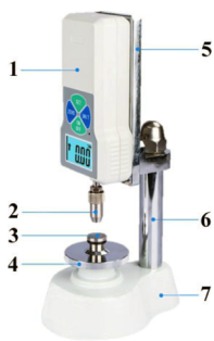
Figure 4. Structure of the digital pressure gauge. 1. Digital operation interface 2. Pressure head 3. Objective stage 4. Hand wheel 5. Adapter plate 6. Column 7. Base.
