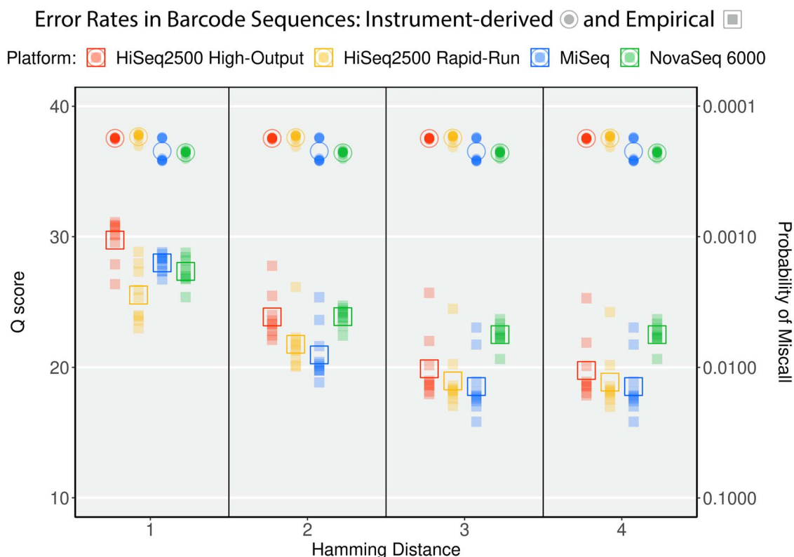
Figure 4. Quality scores from four Illumina platforms measured within barcode regions of reads. The empirical rate of base-calling errors (squares) were sequentially calculated using increasing Hamming distance in the ngsComposer demultiplexing tool, anemone. The Q scores for these bases reported by Illumina software reveal underestimation of base-calling error. Open shapes indicate the mean Q scores, while solid shapes indicate Q scores for individual base positions along the barcode region.
