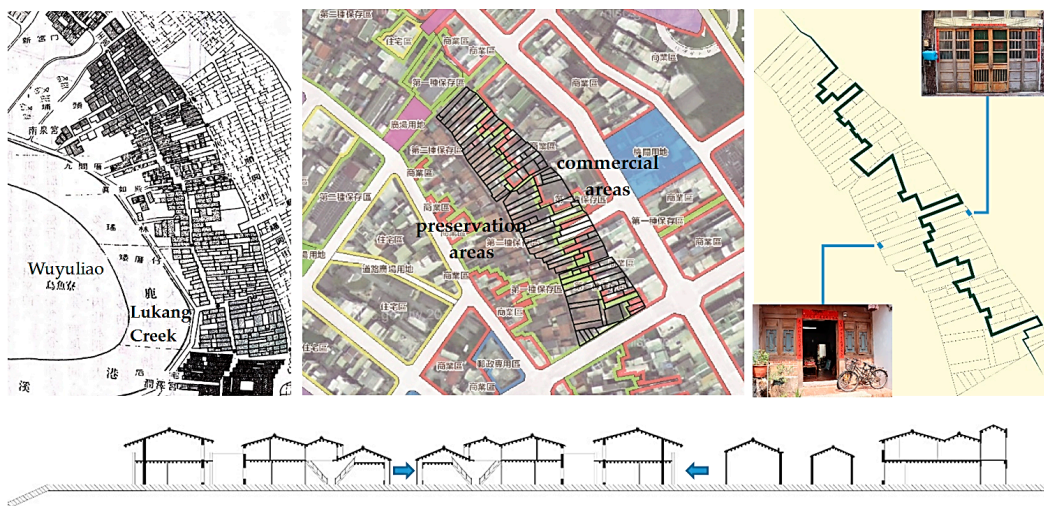
Figure 3. Site plan of the old harbor [57], zoning map, and differentiated street block (top, from left to right); cross section of four streets (bottom).
