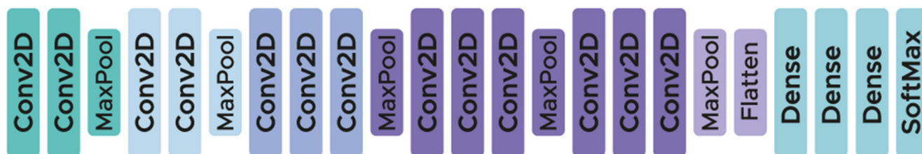
Figure 7. The structure of VGG16.
