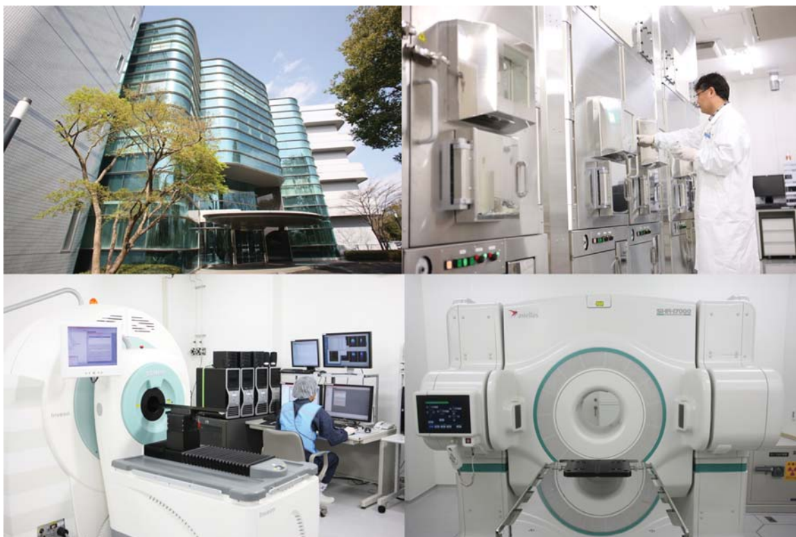
Figure 2. Astellas' Biomimaging Research Laboratories (BIRL). Upper left: Building of BIRL at Astellas Tsukuba Research Center. Upper right: Automated system for PET tracers developed in-house. Lower left: Positron emission tomography (PET)/computed tomography scanner for small animal studies (Inveon, Siemens). Lower right: PET scanner for large animal studies (SHR-17000, co-developed with Hamamatsu Photonics K.K.).
