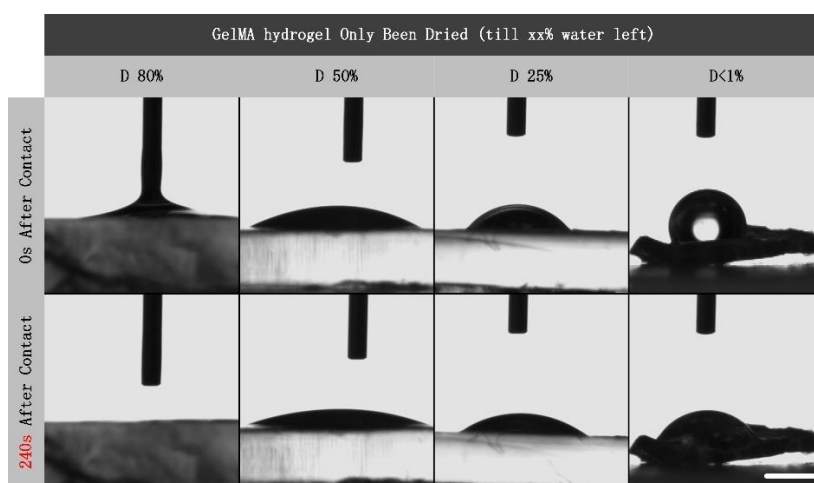
Figure S2. The contact angles of pure water on the dried sample surface. Hydrophilicity is positively correlated with water content. Water droplets can hold for more than 300 s on totally dried surface where water absorption occurs slowly. Scale bar: 500 \mu\text{m} .
