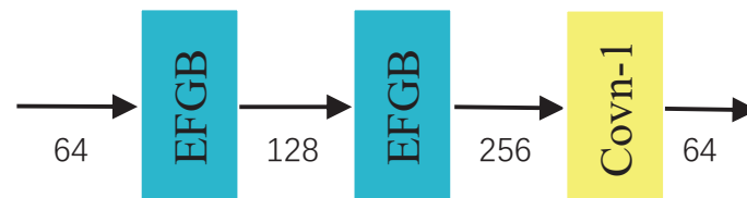
Figure 7. The structure of modified SIRU. 64, 128, 256 represent the channel numbers of feature maps.
