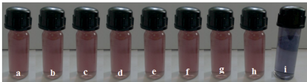
Figure 10. Digital photograph images of AuNPs–rGO composite with the addition of 20 μM of different anions; (a) AuNPs-rGO, (b) F − , (c) Br − , (d) CN − , (e) SO 4 2− , (f) PO 4 3− , (g) C 2 O 4 2− , (h) CO 3 2− and 5 μM addition of (i) NO 2 − .
