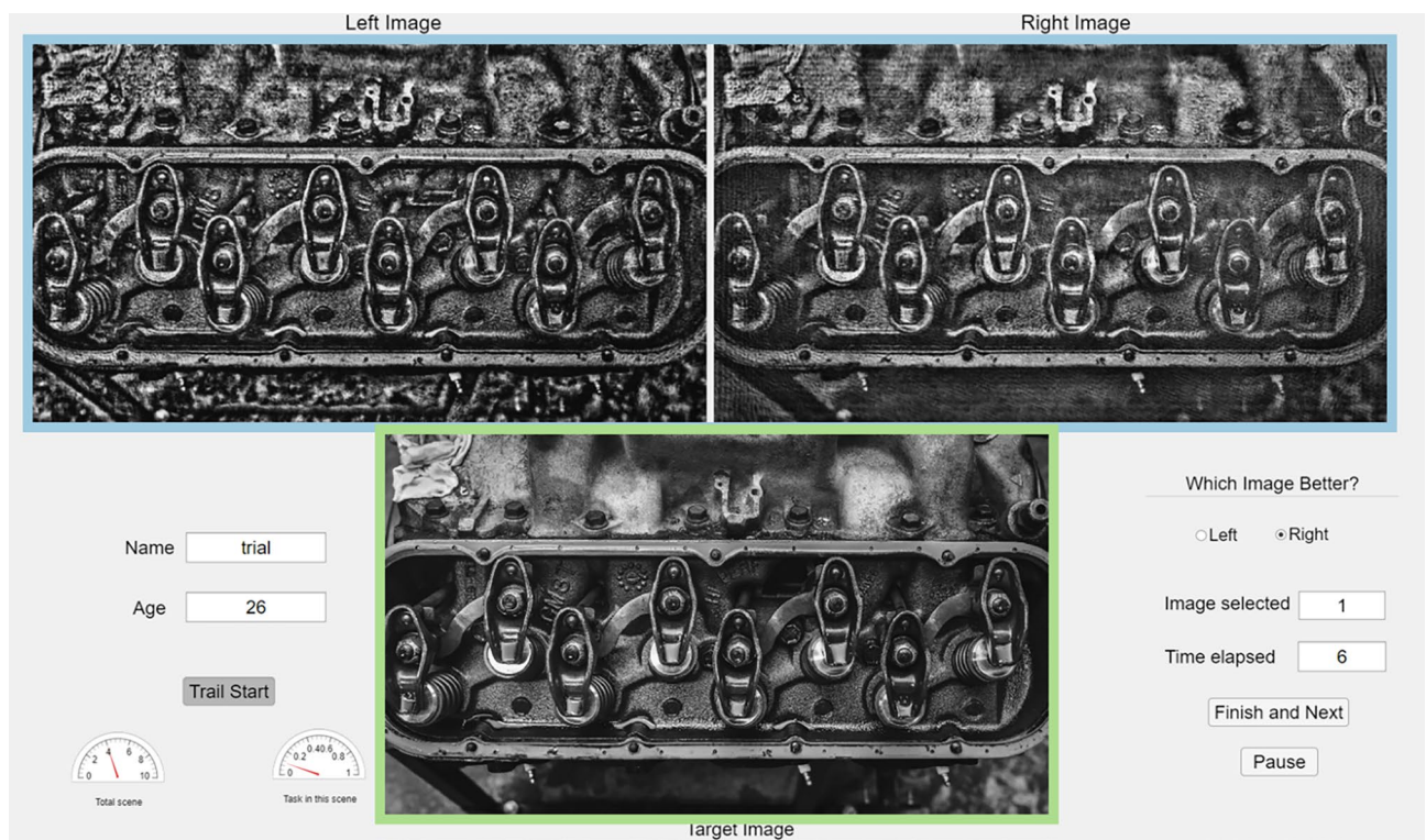
Figure 4. The user interface for collecting human judgments on IQM-based CGH optimization. The experimentally captured image pair from two IQM losses and the corresponding reference image are shown in the blue and the green box respectively.
