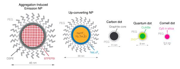
**Figure 1.** Overview of NIR nanoparticles. BTPEPBI: 1,7-tetraphenylethene modified 3,4:9,10-Tetracarboxylic perylene bisimide; Cy5: cyanine 5; DSPE: 1,2-distearoyl-*sn*-glycero-3-phosphoethanolamine-*N*-[amino(polyethylene glycol)]; NP: nanoparticle; PEG: poly(ethyleneglycol).
