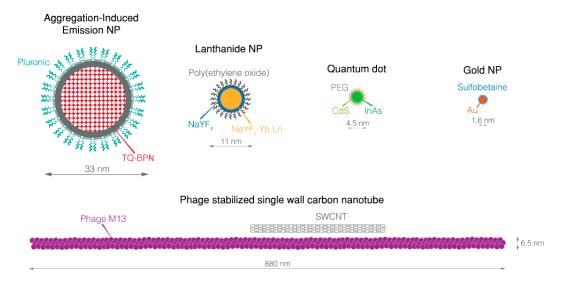
**Figure 2.** Overview of SWIR nanoparticles. NP, nanoparticle; PEG, poly(ethyleneglycol); SWCNT, Single-walled carbon nanotube; TQ-BNP, *N*,*N*′-((6,7-diphenyl-[1,2,5]thiadiazolo[3,4-g]quinoxaline-4,9-diyl)bis(4,1-phenylene))bis(*N*-phenylnaphthalen-1-amine).
