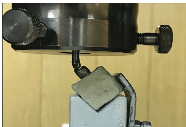
Figure 1: Specimen setting on the universal testing machine.
