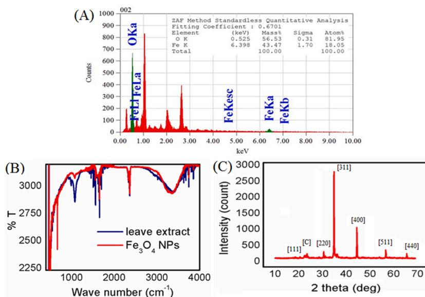
Fig. 4. (A) EDS, (B) ATR and (C) XRD spectra of the synthesized Fe<sub>3</sub>O<sub>4</sub> NPs in PBS buffer pH 7.4 with electrolyte.
