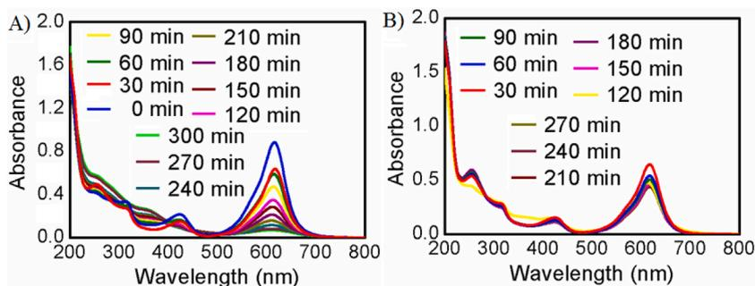
**Fig. 6.** UV–Visible spectra of the 10 mg/L MG in water after adding 1 mg/mL synthesized  $\text{Fe}_3\text{O}_4$  NPs as adsorbent for a period of time in (A) UV light irradiation condition and (B) room light condition respectively.
