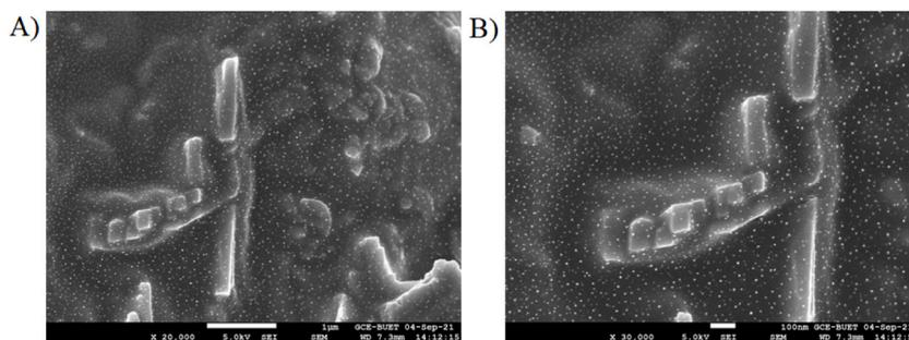
**Fig. 3.** SEM images of the synthesized  $\text{Fe}_3\text{O}_4$  NPs as (A) 1  $\mu\text{m}$  scale bar with  $\times 20,000$  magnification and (B) 100 nm scale bar with  $\times 30,000$  magnification in PBS buffer pH 7.4 with electrolyte.
