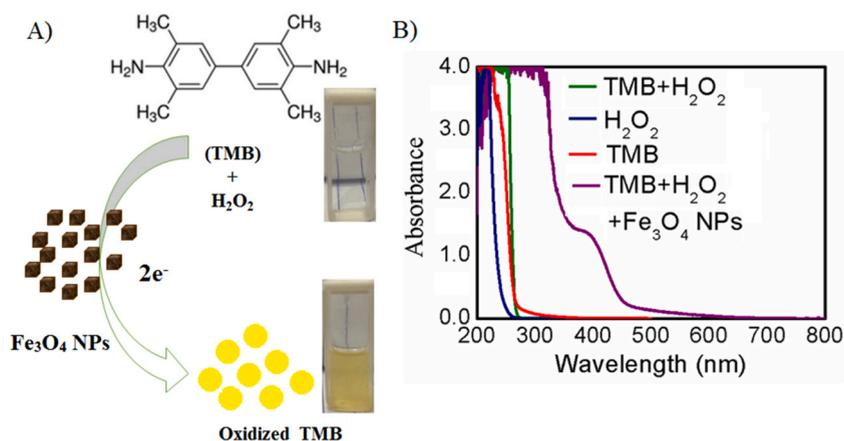
Fig. 5. (A) Schematic representation of TMB oxidation by H<sub>2</sub>O<sub>2</sub> and Fe<sub>3</sub>O<sub>4</sub> NPs as peroxidase enzyme and (B) UV-Visible spectra of the synthesized Fe<sub>3</sub>O<sub>4</sub> NPs in PBS buffer (50 mM) pH 7.4 with 0.00208 M TMB (in acetate buffer pH 4.5), and 0.1 M H<sub>2</sub>O<sub>2</sub>.
