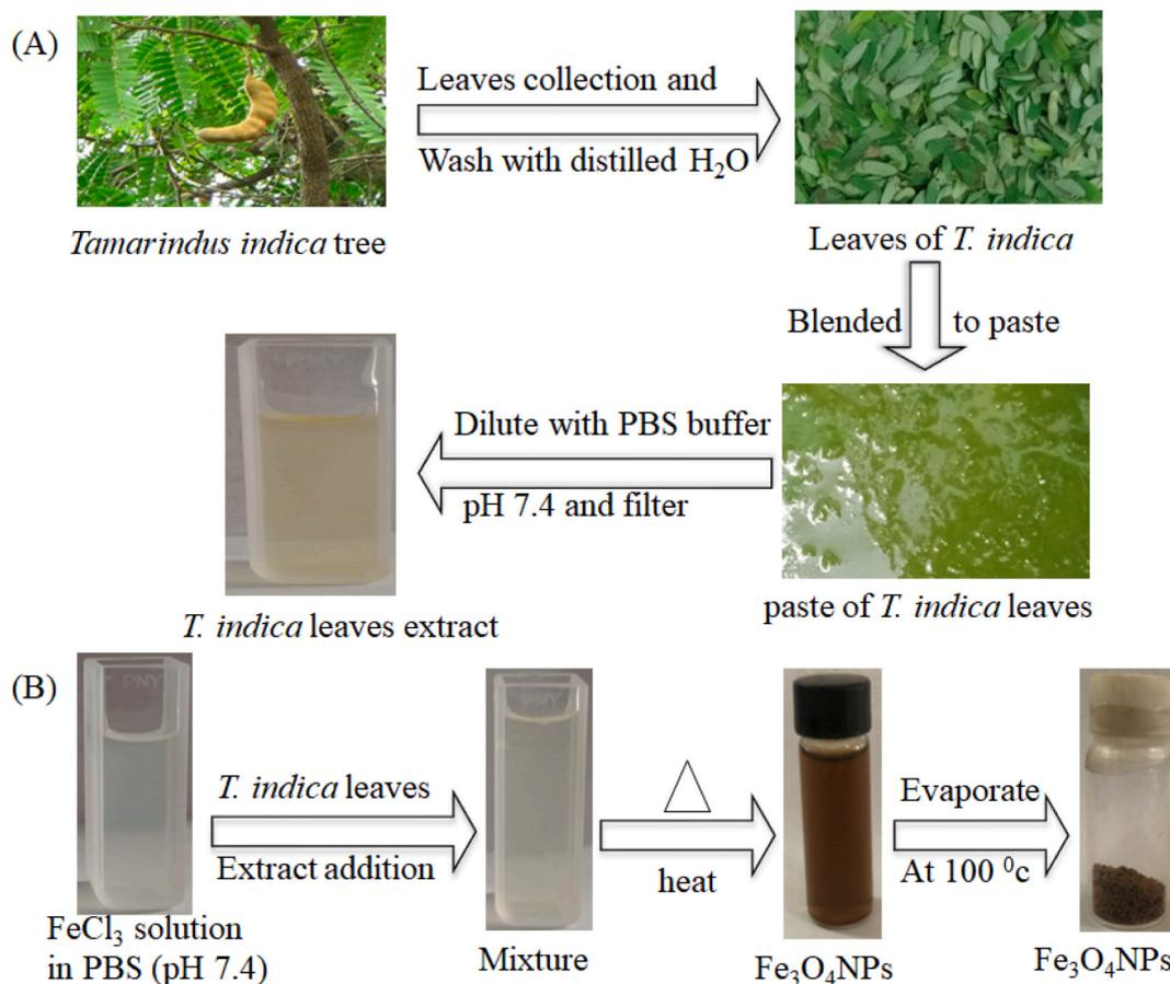
**Scheme 1.** Schematic representation for the (A) preparation of *T. indica* leaf extract and (B) synthesis of  $\text{Fe}_3\text{O}_4$  NPs from *T. indica* leaf extract.
