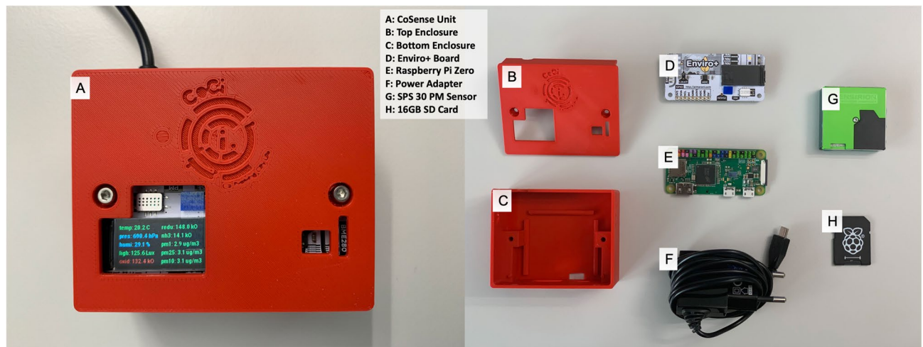
Figure 4. A complete and exploded view of the CoSense Unit with annotations.
