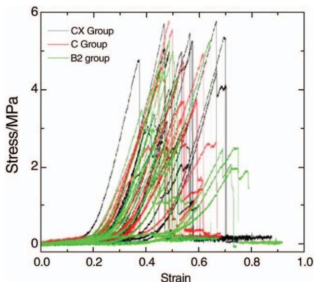
Figure 2. The stress–strain curves of the three groups.
