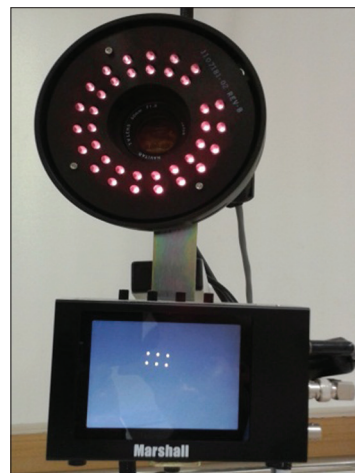
Figure 1: Camera system with infrared illuminator (wall-mounted) and display unit. Marker dots are seen in the monitor
