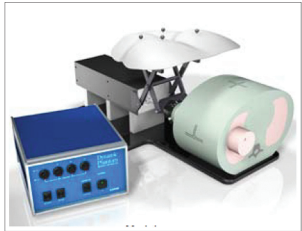
Figure 4: Computerized Imaging Reference Systems dynamic thorax phantom; (lung equivalent, actuator [black box], controller [blue box])
