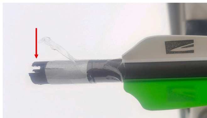
Fig. 5. Photograph of the fragmented “nock” (arrow) from the Killer Instinct DeadStop™ Decocking Bolt used at the time of trauma.
