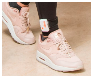
Figure 2. Placement of the Inertial Measurement Unit (IMU) on the lateral side of the ankle, above the malleoli.
