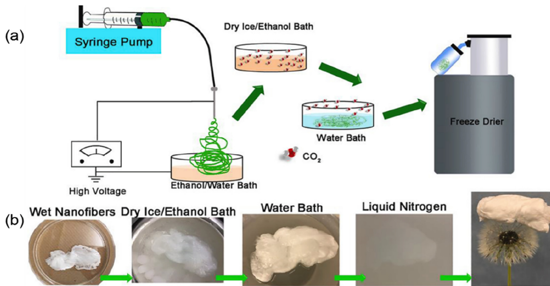
Fig. 4. (a) Schematic to fabricate 3D nanofibrous scaffolds. (b) Representative photographs of the electrospun nanofibers in each step during the fabrication process. Reprinted with permission from Ref. [38].
