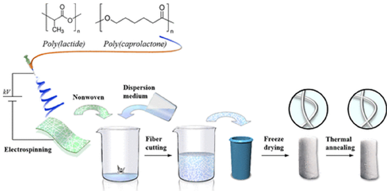
Fig. 10. Schematic to illustrate the general sponge fabrication steps. Reprinted from Ref. [48].
