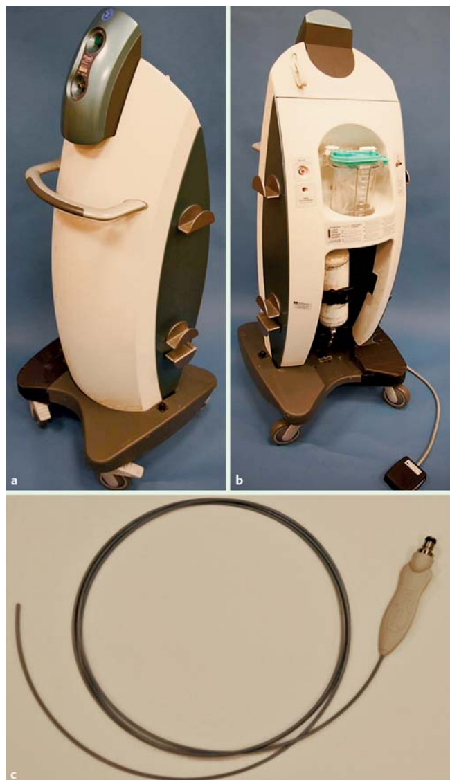
Fig. 1 The Polar Wand CO 2 cryotherapy system. a The front of the portable system. b The tank with the compressed CO 2 gas and the disposable suction bottle at the back of the system, and the foot pedal to apply the gas flow. c The 7-French flexible cryospray catheter, which is introduced through the working channel of the endoscope.
