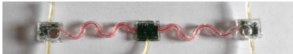
Figure 14. Final sensor: the three subparts (left sEMG, main unit and right sEMG) packaged in PDMS with the two batteries included. Vertical wires are connected to electrodes.
