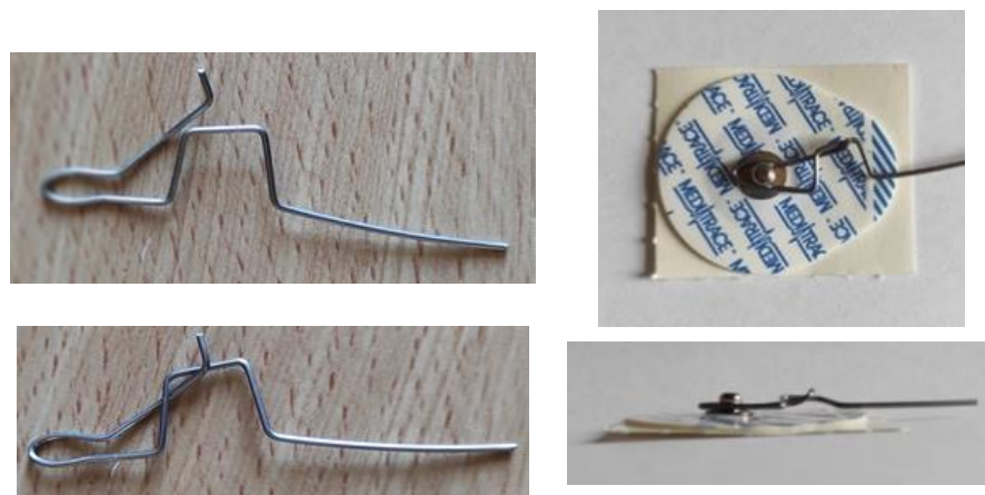
Figure 15. Thin clamping system developed to connect the electrode to the sensor without affecting the final thickness.
