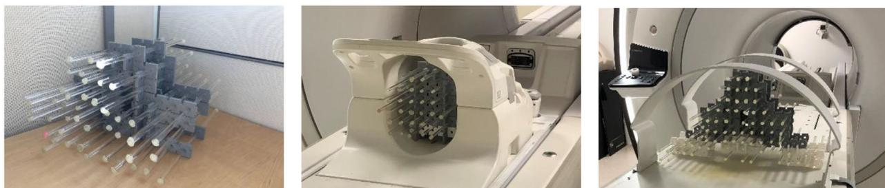
**FIGURE 2** (a) The phantom made of assembled plastic blocks and glass tubes filled with water, (b) assembled phantom that fits the head coil, and (c) assembled phantom that fits the anterior coil
