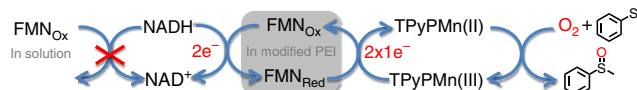
Figure 10 | Schematic representation of the complete catalytic system. The artificial flavoenzyme collects electrons from NADH and provides a single-electron flow to the Mn(III) porphyrins to activate dioxygen and perform catalytic oxidation in water.
