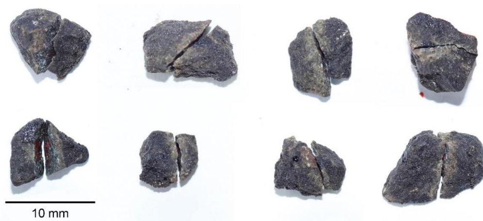
Figure 17. Aggregate fracture location distribution.
