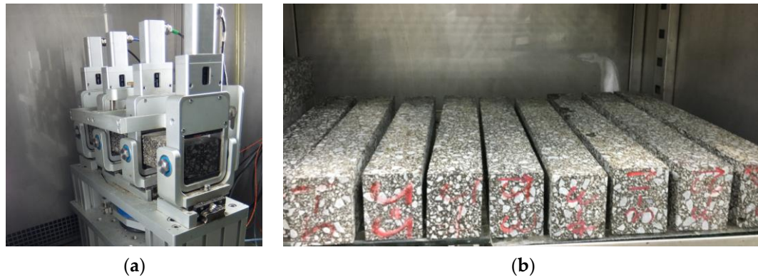
Figure 7. The test device and beam specimens: (a) four-point bending fatigue device and (b) EAC beam specimens.
