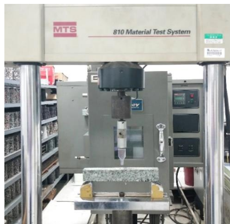
Figure 4. Three-point bending test device for the epoxy asphalt mixture beams.
