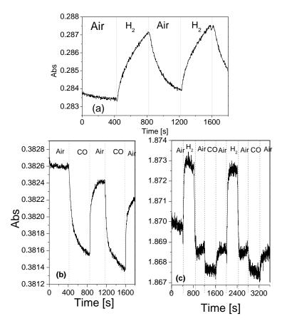
The dynamic responses at 650 nm for CO and at 340 nm for H<sub>2</sub> and CO are plotted in Figure 9b,c, respectively. The response time for CO at 650 nm is about 300 s, but at 340 nm response time is reduced down to 40 s. Dynamic resistance measurements of Fe activated WO<sub>3</sub> films for CO sensing at 423 K,
