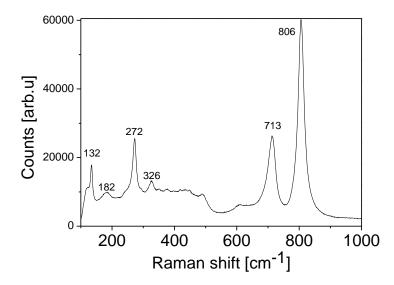
Figure 2. Raman spectra of the TO film annealed at 973 K.
