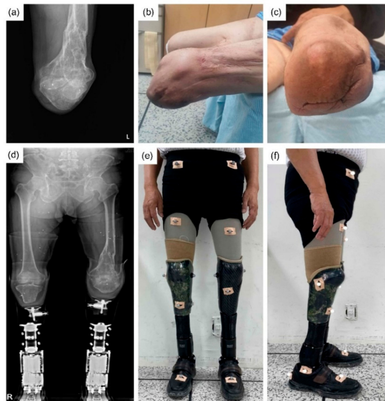
Figure 1. (a) X-ray of left knee flexion contracture due to distal femur malunion. (b) Flexion contracture of 10^\circ of the left leg. (c) Cylindrical left stump with intact soft tissue shrinkage in healing state. (d) Lower extremities X-ray view with RoFT ® . (e,f) The front and side view of participant wearing RoFT ® . 19 sensors attached with the Helen-Hayes method to the anterior superior iliac spines, sacrum, thighs (midpoint between the greater trochanter and the lateral femoral head), knee joint, tibial tuberosity, ankle medial and lateral malleolus, heel, and second metatarsal bone. With bilateral prostheses, it is difficult to attach sensors in the correct anatomical position.
