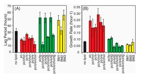
**Figure 3.** Plot of the lag periods ( $t_{lag}$ , **A**) and growth rate constants (k, **B**) for A $\beta_{40}$  fibrillization in different membrane models. Error bars were generated from three repetitions of thioflavin-T (ThT) kinetic curves shown in Figure 2. Different colors are used to facilitate the presentation (different model membranes).
