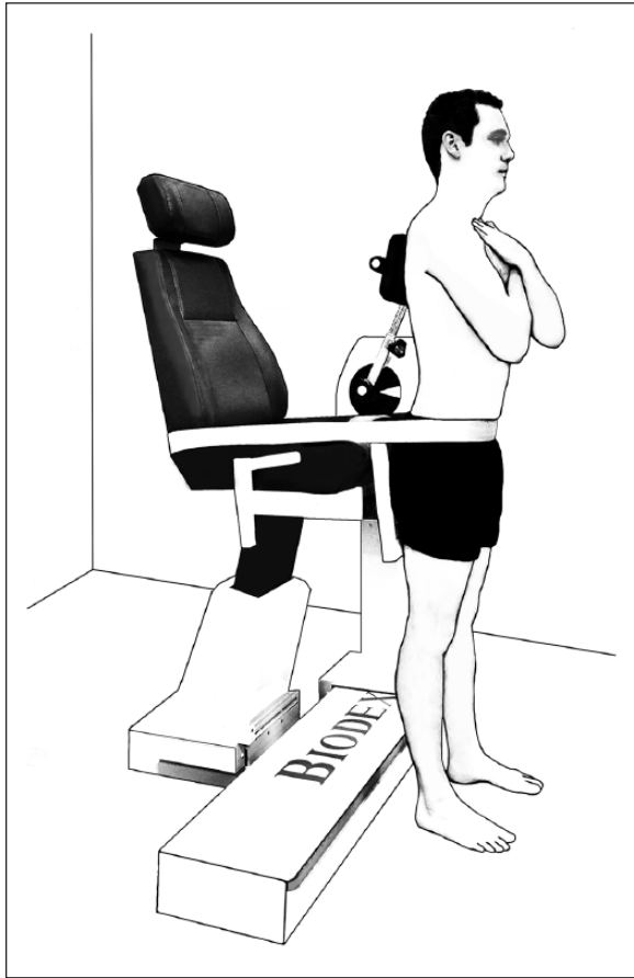
Figure 1. Participant and dynamometer positioning for isometric back extensor strength measures with the isokinetic dynamometer.
