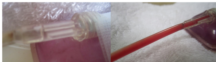
Figure 4 Post treatment clot constituent mixing (Control vs. LFVP sample). Image (left) shows the typical (and absent) degree of post treatment dissolved clot constituent mixing into the connecting line of a control sample (from sample no. 9). Control samples never at any time showed any permeation of red color into the connecting line. Image (right) shows the comparatively pronounced degree of mixing commonly observed in a LFVP sample (image taken from sample no. 10).
