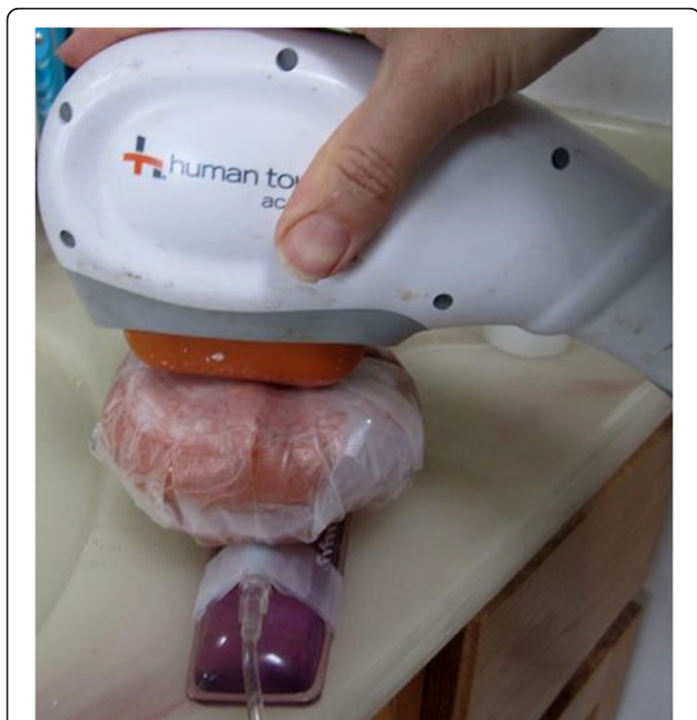
Figure 1 Our vibration set up. A 50 Hz massager was intermittently engaged upon a 4 cm thick meat slab overlying our clotted catheter segment. Visible is the pressurized connecting line protruding from underneath the slab. Not seen (under the slab) is the capped, 4 mm lumen Soft Flo Catheter segment with indwelling clot. To view the application in real time, please refer to the following internet link: http://www.youtube.com/watch?v=6ClcDttuERA .
