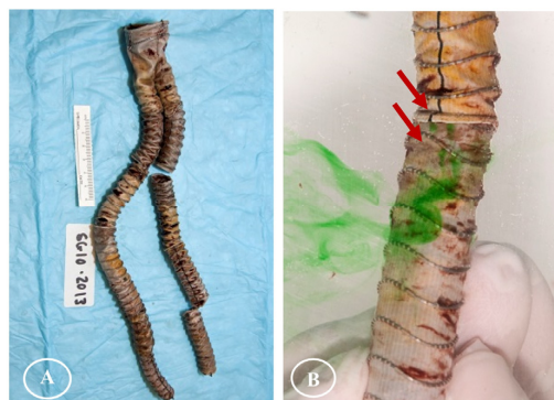
Figure 3. Deformation from twisting in the body of an explanted Anaconda device is maintained after explantation. The fabric preserves its imperviousness according to the gross observation (A). However, endoleaks were shown in the distal limb (B).
